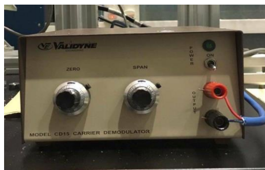
Figure 2-27 Validyne DP15 pressure transducer Figure 2-28 Validyne CD15 Carrier Demodulator
