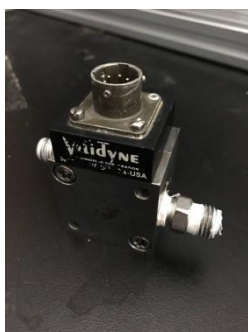
Figure 2-27 Validyne DP15 pressure transducer Figure 2-28 Validyne CD15 Carrier Demodulator
