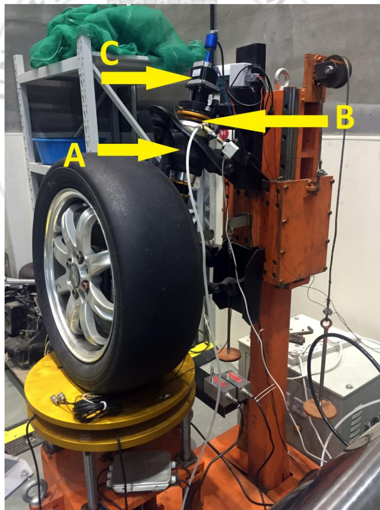
Figure 4.4 Overview of the quarter car test rig with sensors
