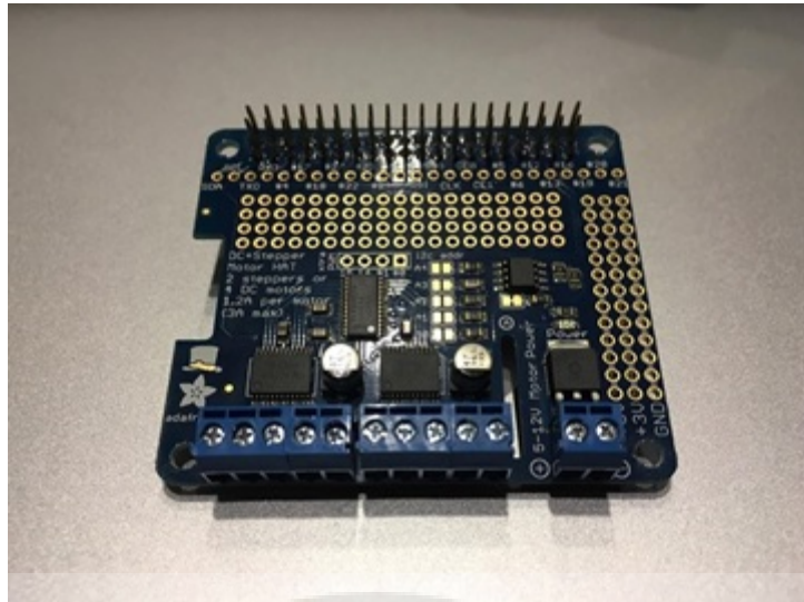
Figure 2-9 Adafruit DC and Stepper Motor HAT
