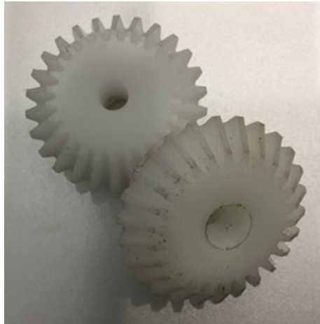
Figure 2-14 Nylon bevel gears
