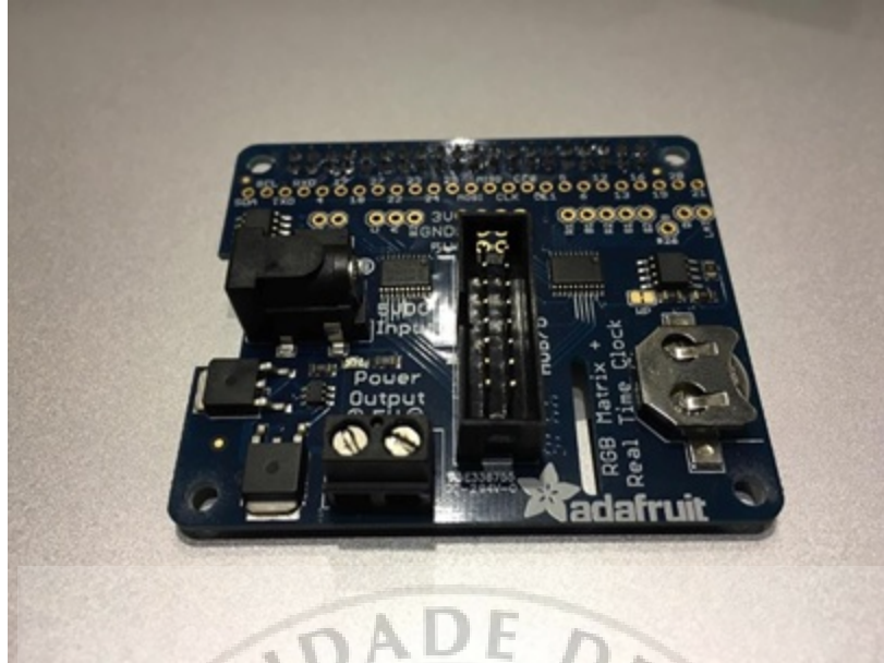
Figure 2-7 Adafruit RGB Matrix + Real Time Clock Hat
