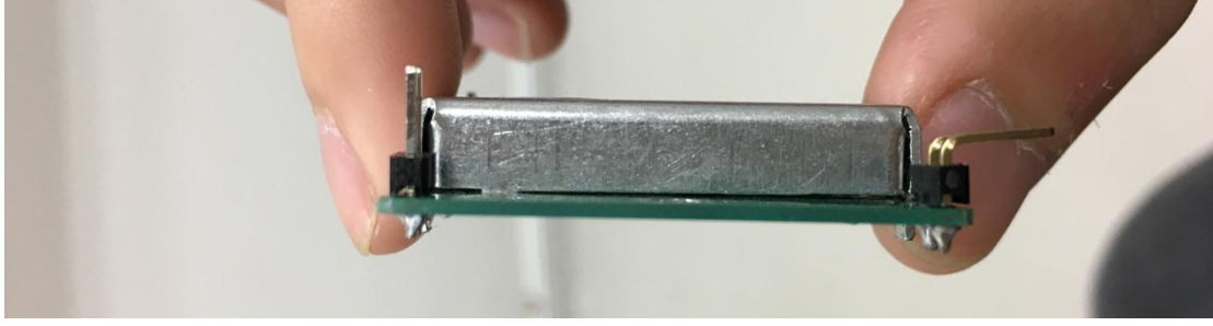
Fig 3. 4 The side face of HB100, we can see the back has a metal cover which can reduce external distortion.
